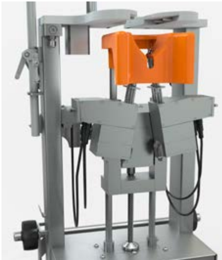
Up to five synchronously operating vaccination needles reduce the stress during the vaccination process for the pullets
