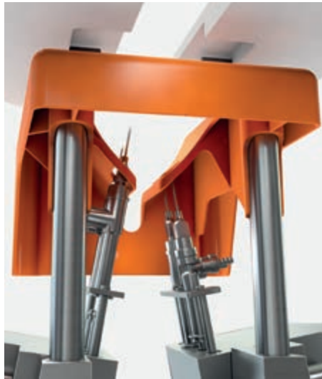
Up to five synchronously operating vaccination needles reduce the stress during the vaccination process for the pullets
